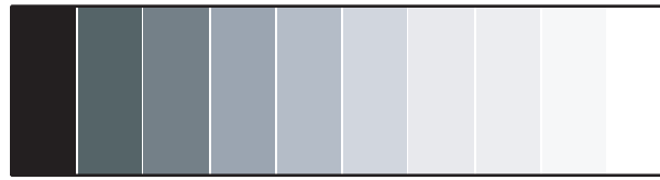
Figure 4-10: Typical Gray Bar Pattern for Adjusting Contrast
